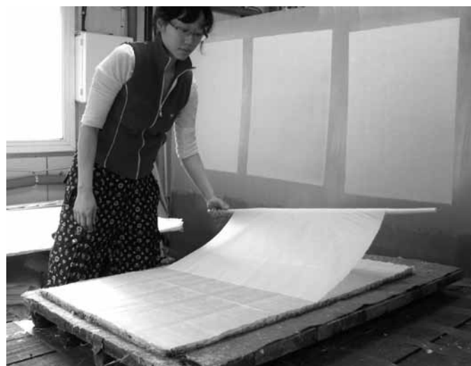
The author uses the stripped woody core of a dak branch to part a sheet of hanji from a pressed post of formed paper. She will brush the sheet on the heat dryer behind her.
