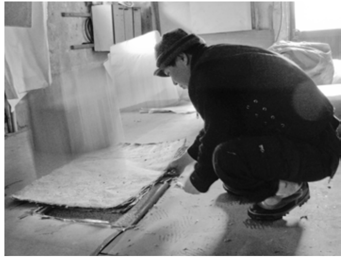
Jang Seong-woo uses a homemade device to hammer hanji made of white, green, and black bark. The paper was dried and then slightly dampened before being calendered in a method called dochim, used in Korea to compact fibers, increase sheen and strength, and prevent excessive ink bleed.
