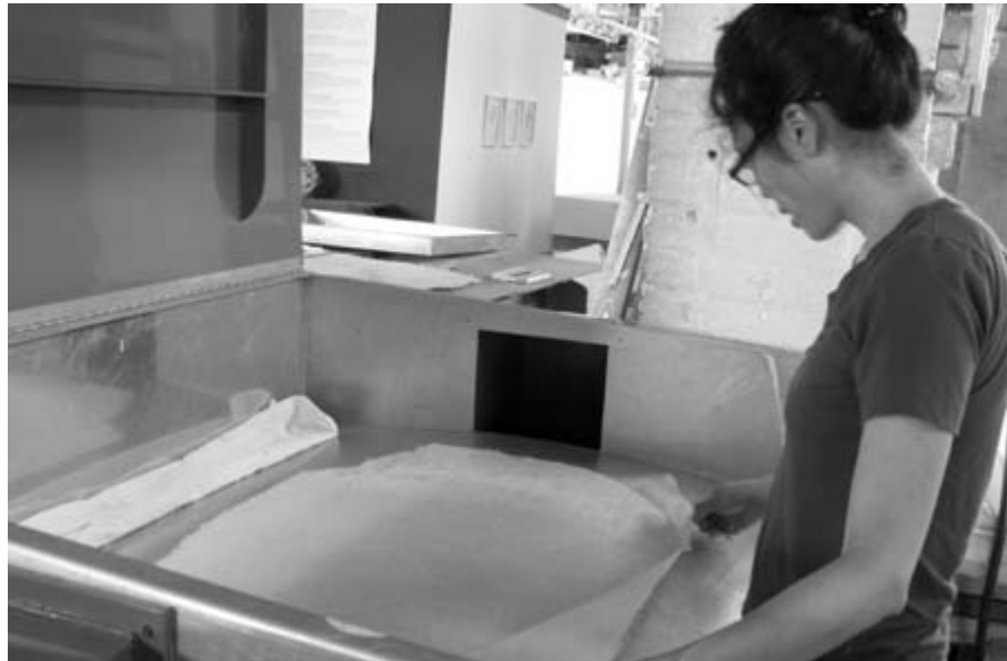
Aimee Lee peels away a dry sheet of hanji from the curved surface of the heat dryer. The steel plate is heated while a dehumidifier removes moisture from the sheet. The system circulates air through the wide plastic passage that opens to the right and left of the steel plate. Photo: Stephanie Brewer.
