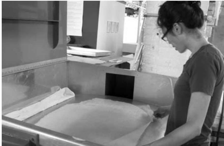
Aimee Lee peels away a dry sheet of hanji from the curved surface of the heat dryer. The steel plate is heated while a dehumidifier removes moisture from the sheet. The system circulates air through the wide plastic passage that opens to the right and left of the steel plate. Photo: Stephanie Brewer.
