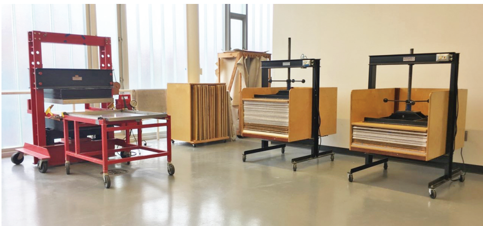
Fig. 27b. The second hydraulic press and two dry boxes by Reina at Longwood University. Photograph courtesy Kerri Cushman.
