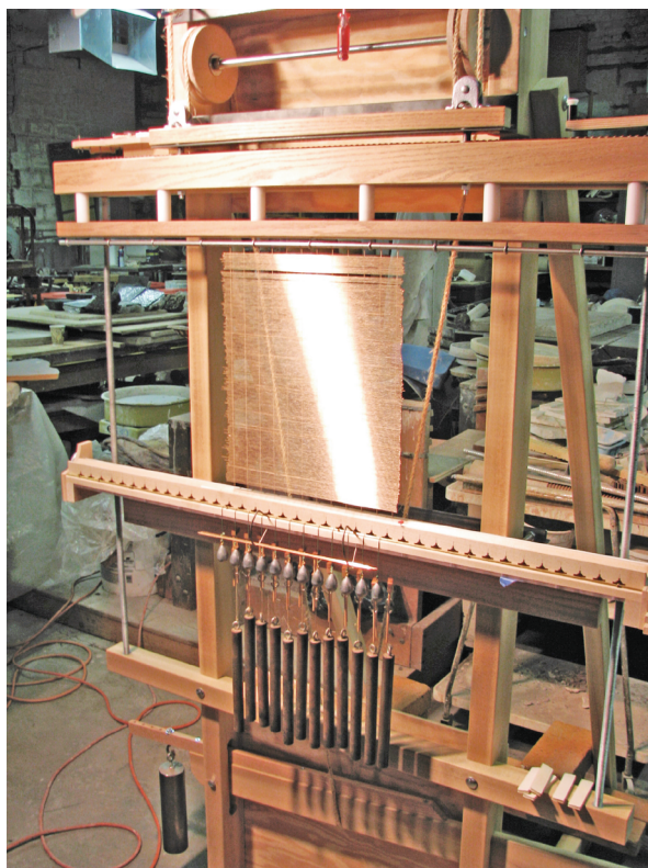
Fig. 5. Loom for weaving mould facings by Moore set up in Cleveland, Ohio, at Tom Balbo's private studio for teaching pre-conference workshops at the 2012 joint meeting of the Friends of Dard Hunter and the International Association of Hand Papermakers and Paper Artists (IAPMA).
