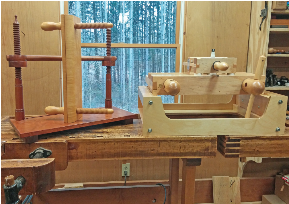
Fig. 9. Some of Moore's bookbinding tools, including a sewing frame and finishing press (left) and compact lying press with plow on top (right). December 2017.
