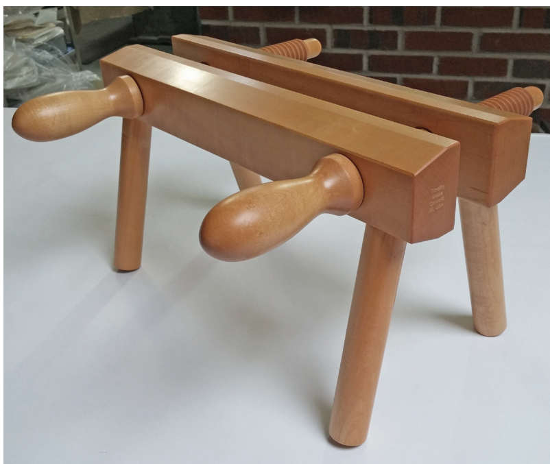
Fig. 7. Moore's repair press. This is the smaller version on shorter legs. A taller version accommodates wider books. December 2017.
