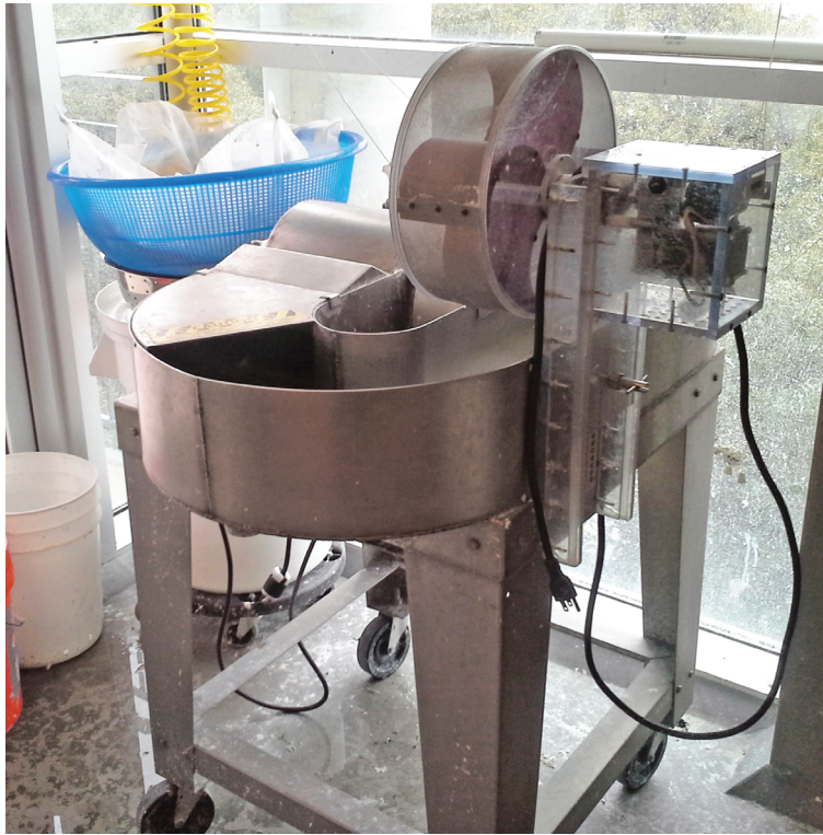
Fig. 25. Reina two-pound beater with washer at Trinity University; papermaking studio set up by professor Jon Lee. February 2012.
