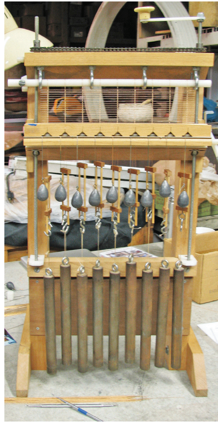
Fig. 11. Moore's loom for miniature mould facings. Set up at 2012 joint meeting of the FDH and IAPMA.
