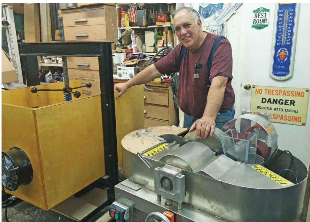
David Reina with new dry box (stack dryer) and two-pound beater in his shop. May 2017.
