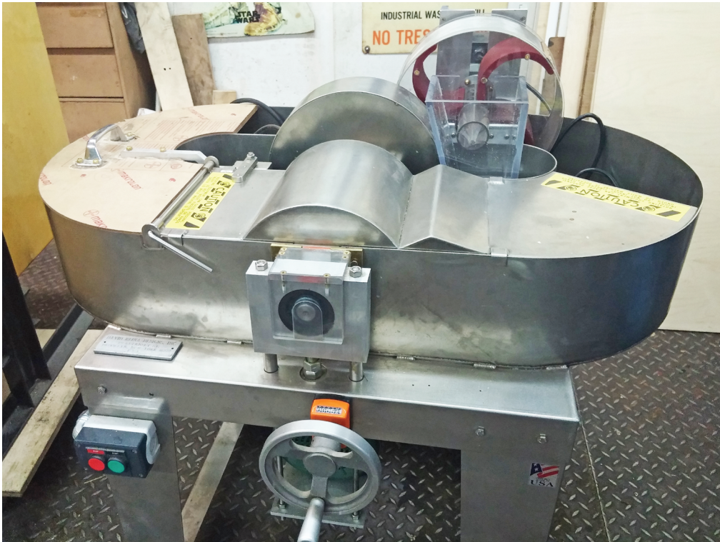
Fig. 2.4. Reina two-pound beater with new counter mechanism. May 2017.
