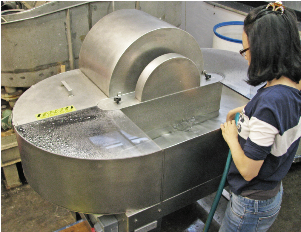
Fig. 31a. Lee fills naginata with water at the Morgan Conservatory in Cleveland; note similarities in design to Reina's Hollander beaters. August 2014.
