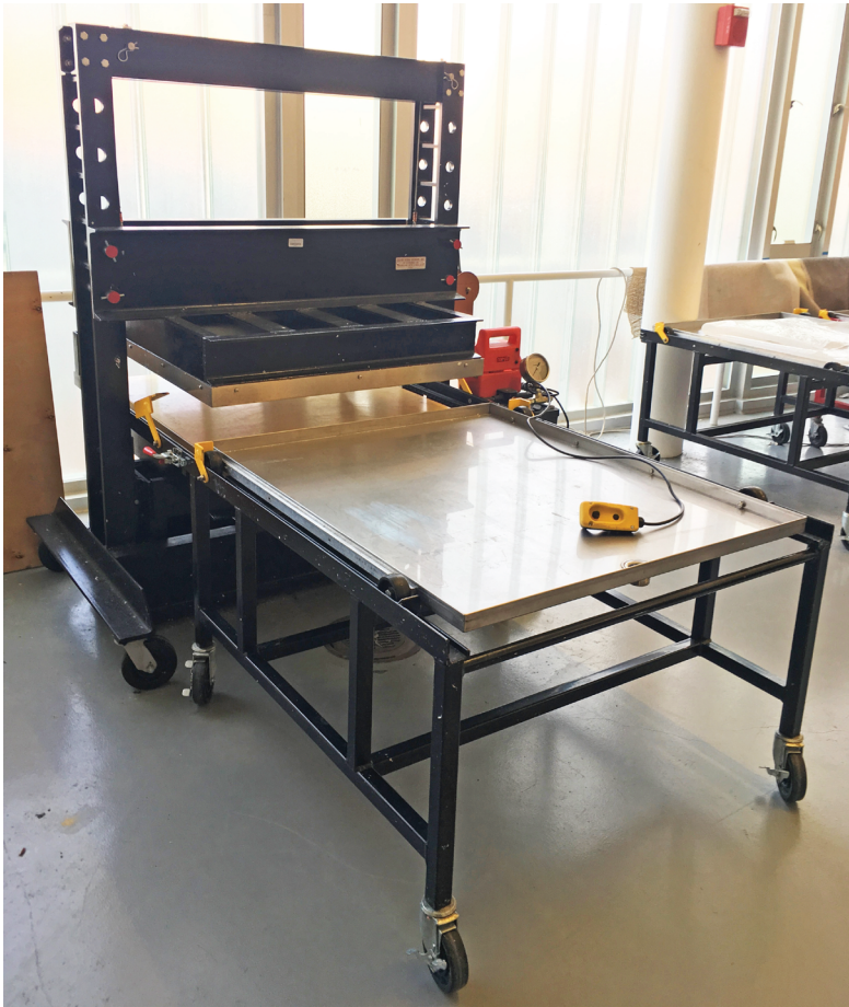
Fig. 27a. One of two hydraulic presses with couching table by Reina at Longwood University. Photograph courtesy Kerri Cushman.
